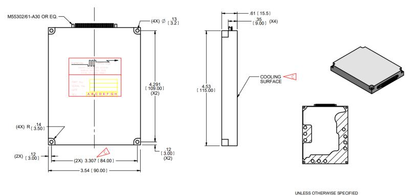
DIMENSIONS ARE IN INCHES (MM). TOLERANCES ARE: DECIMALS ANGLES .XX± 0.02 .XXX± 0.010 DO NOT SCALE DRAWING ±
