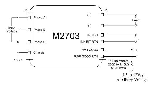
**Note:** PWR GOOD pull-up resistor and auxiliary voltage shown in this diagram are typical values. The system designer must select the actual values such that no damage can occur to the internal components of the power supply *– consult factory for more information*.
