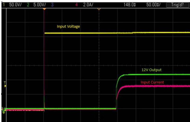
Figure 3.5.1.6-2 Outputs Turn-on Inrush. <0.1A Input Inrush current with 12V Loaded.
