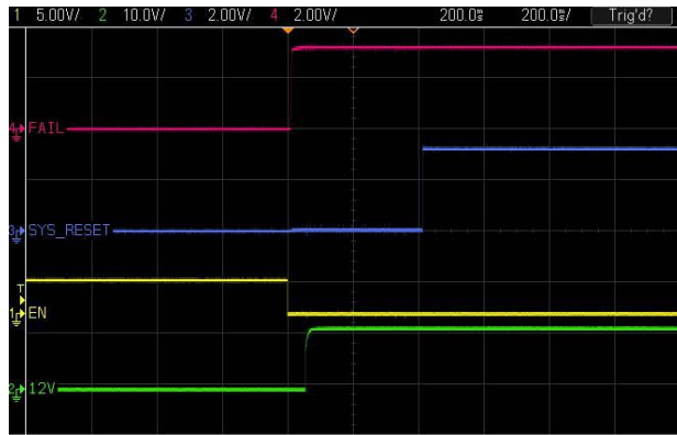
Figure 3.5.3.2-3 BITs status Enable Turn-on
